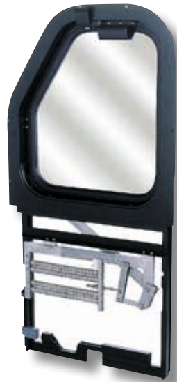
Spring-assisted drop window Bombardier
